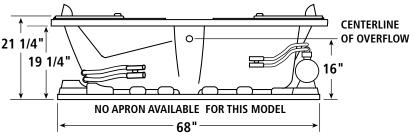
**DRAIN AND OVERFLOW** DRAIN CUTOUT = 2" OVERFLOW CUTOUT= 2 1/2"
