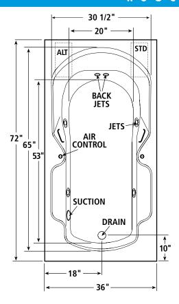
**NOTE:** Rough-in measurements may vary 1/4" (+/-). Pump locations are shown for clarity. STD-standard pump location. ALT-optional alternate pump location. \*\* Electronic SimpleSelect located on (Std or Alt) corner of deck.
